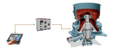
To resolve this issue, Minprovise have a system that automatically analyses the crusher product belt and provides documentable numerical data reflecting crusher performance based on current feed ore characteristics, enabling a real-time adjustment to ensure optimal production. The system requires no manual intervention and accommodates not only feed material property changes but also crusher liner wear profile variances.
